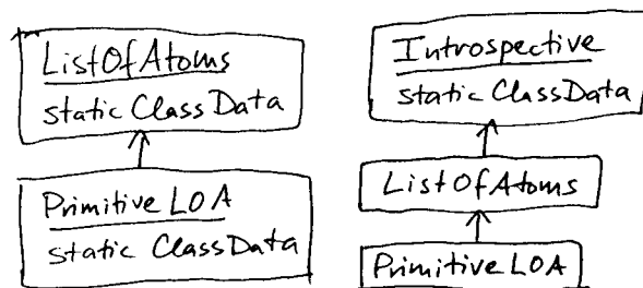
Figure 3: There are two ways to picture placing static class data in an object. A separate structure for each class makes communication among classes difficult while using a single static store in a base class replicates the functions of a Meta-Object Protocol in a less plastic configuration.
