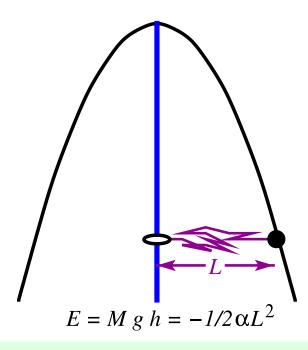
Rubber band stretched by weight on a hill. We place the endpoint of the spring (disk at L) in a parabolic potential– $(1/2)\alpha L^2$ , as suggested by this schematic diagram.
