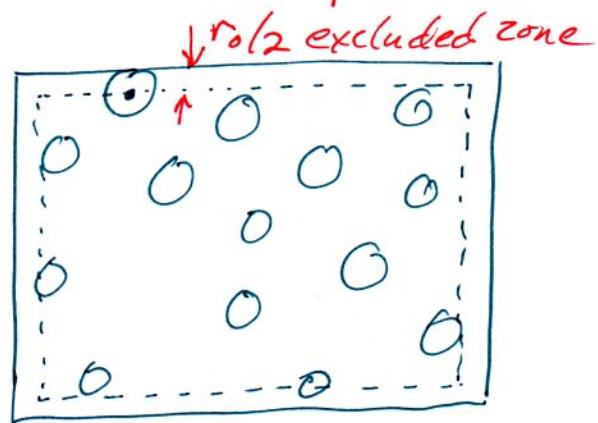
$$\rho(\vec{r}) = \frac{1}{(L-r_0)^3} = \frac{1}{V} \text{constant away from the sides of the box, for a dilute gas}$$
