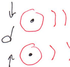
Multiple sources of waves, spaced by  $d$
