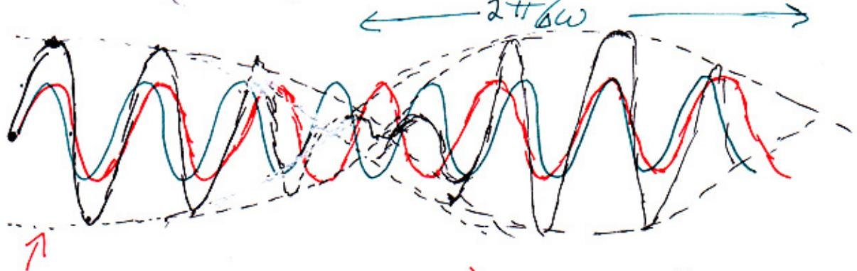
$$\text{Envelope} = \pm 2 \cos\left(\frac{\Delta\omega t}{2}\right) \quad (\text{Smooth curve over wiggles})$$
