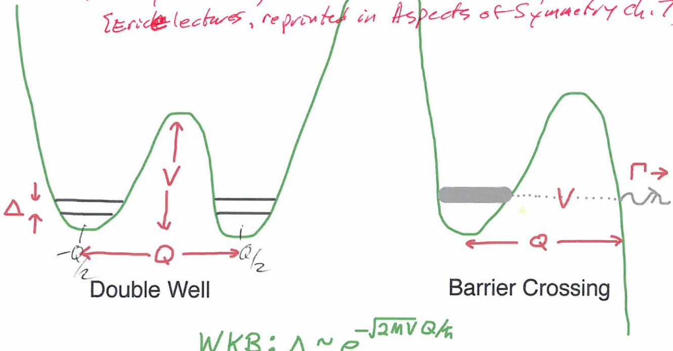
$$WKB: \Delta \sim e^{-\sqrt{2mV}Q/\hbar}, \quad \Gamma \sim \Delta^2$$
