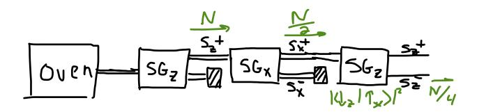
Half of the original sz+ particles removed by second block Fraction of Sx+ beam now Sz- is  $|\langle \downarrow_z \rangle|^2 = \langle \downarrow_z \rangle$
