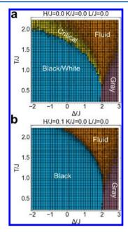
**Figure 5.** Cross sections of the phase diagram for the Blume-Capel model (K = 0, L = 0), with H/J = 0 or 0.1. Colors have the same meaning as in Figure 3.
