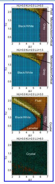
**Figure 4.** Cross sections of the phase diagram at varying values of the surfactant strength. Surfactant strength L/J is varied from 0 to 6, with constant H/J = 0, K/J = 2. Colors have the same meaning as in Figure 3.
