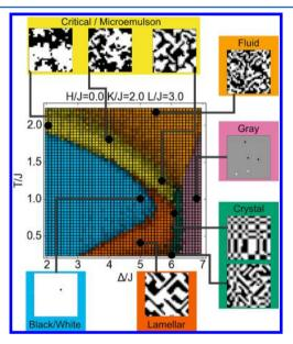
Figure 3. Phase diagram of the lattice model. The color of each pixel with specified  $(\Delta/J, T/J)$  coordinates indicates the phase at that point, as determined by the neural network. Pixels with a higher brightness indicate a higher level of confidence in the classification. Snapshots show typical examples of each of the phases, corresponding to the black points on the phase diagram.
