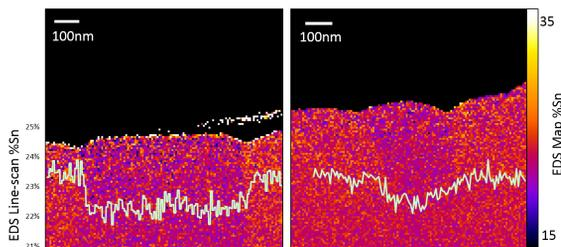
Figure 6: An EDS map of two grains on the surface of the  $Nb_3Sn$  layer, seen in a cross-section view by TEM. Superimposed on the grains are linescans giving a more detailed observation of the atomic-% Sn content in the grain relative to its neighbours.
