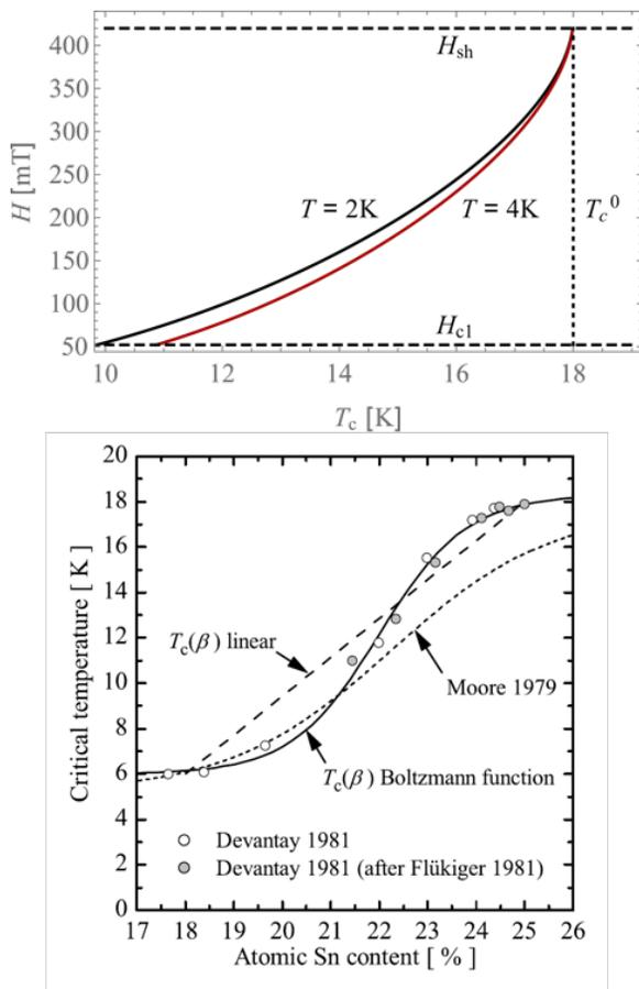
Figure 5: (Top) Calculations of the flux entry field as a function of the  $T_c$  suppression in the first 100 nm of the RF surface and (Bottom) the dependence of the  $T_c$  on the atomic-% Sn [7].
