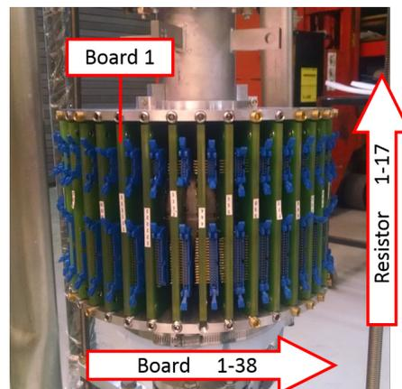
Figure 1: The single-cell temperature mapping system in use at Cornell University, mounted onto a 1.3 GHz single-cell ILC-style cavity coated with Nb<sub>3</sub>Sn. The cables connecting the boards to the data acquisition system have been removed for better visibility.
