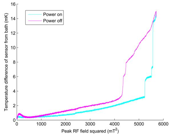
Figure 4: A plot of the  $\Delta T$  of the sensor at the quench origin with respect to the bath versus the square of the RF magnetic field in the cavity. In this plot, Ohmic losses appear as a linear dependence. The cyan line is data obtained as the cavity powered up, while the magenta line was obtained as the cavity was allowed to ring down.
