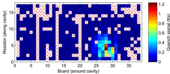
Figure 2: A quench map of the cavity, indicating the location of the quench. The quench map integrates with respect to time the temperature of the sensor after the quench is detected on the RF signal. Regions that remain hotter for longer indicate a sensor closer to the quench origin. A red cross indicates a non-responsive sensor.
