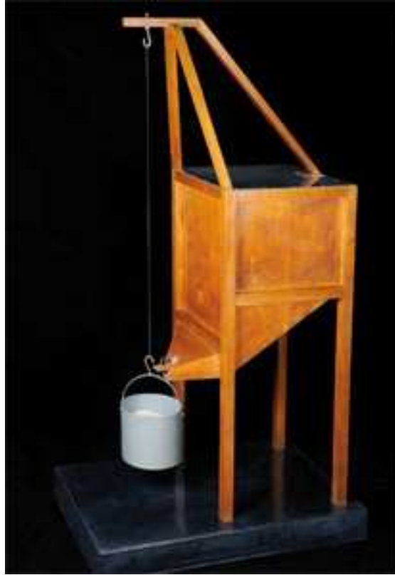
Figure 1.1: A reproduction of Leonardo da Vinci's experimental apparatus for testing the tensile strength of wires of varying length and thickness, based on his drawings in his notebook Codex Atlanticus , sheet 222 1486-1490. The apparatus consists a container to hold sand, and pour it slowly into a bucket suspended by a wire. The weight of sand at which the wire broke would characterize the strength of the wire. Image copyright: 2013 Museo Nazionale della Scienza e della Tecnologia "Leonardo da Vinci" all rights reserved.
