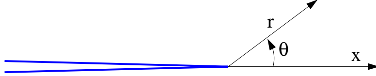
Figure A.1: Polar coordinates at a sharp crack tip. The \theta = 0 direction is aligned with the crack, while \theta = \pm\pi gives the two crack surfaces that are assumed to extend indefinitely (marked in bold blue color).
