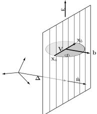
FIG. 2. The orientation of the plain is defined by the vector normal  $\hat{\mathbf{n}}$ . The Rodrigues vector  $\boldsymbol{\omega}$  gives the axis of rotation and the angle of relative orientation between the two grains across the boundary.
