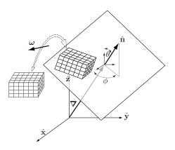
FIG. 1. A general grain boundary whose normal is  $\hat{\mathbf{n}}$  positioned at the distance  $\boldsymbol{\Delta}$  away from the origin separates two unstrained regions with a relative orientation defined by  $\boldsymbol{\omega}$ .
